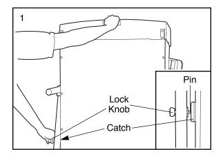
2. Hold the treadmill firmly with both hands, and lower the treadmill to the floor. To decrease the possibility of injury, bend your legs and keep your back straight.
